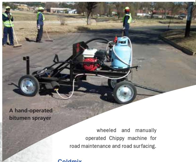
A hand-operated bitumen sprayer
